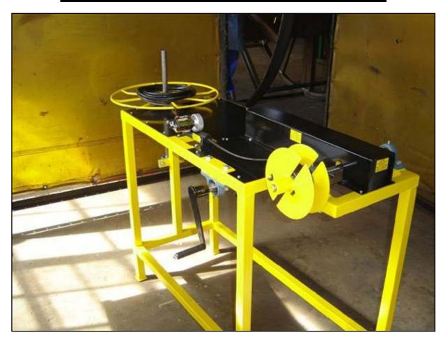
The bench coiling machine was first designed for the packing industry. This machine is ideal for decoiling small lengths from a 100 meter coil and can also accept drums. This machine is capable to coil any form of flexible tubing, rope, hose etc.
